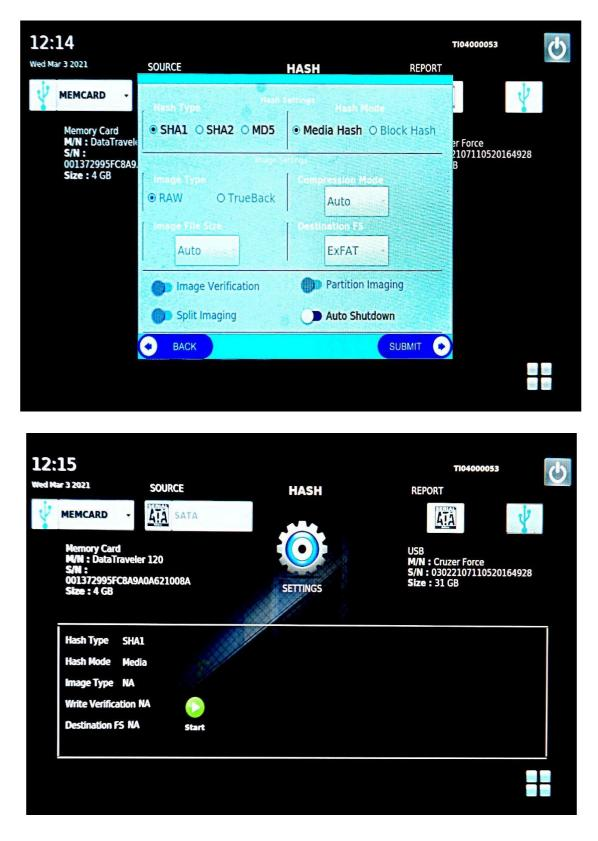
**Step 4**: Click Hash button. Now Hash process screen will be displayed. Select Source disk interface type from Source combo box.
