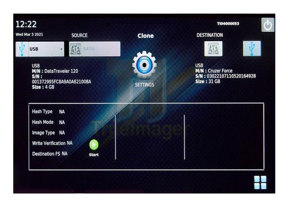
Step 8: Switch of the unit by clicking the Power OFF button. The destination disk will now have all the files as in source disk.
