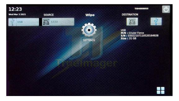
Step 3: Click Wipe button. Now Wipe process screen will be displayed. Select Destination disk interface type from Destination combo box. Now Destination disk details will be displayed.
