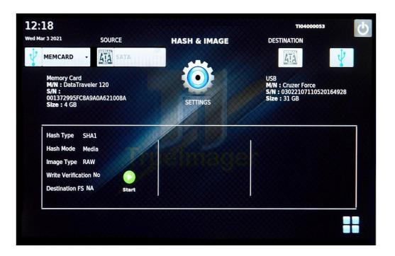
**Step 5:** Select Destination disk interface type from Destination combo box. Now Destination disk details will be displayed.
